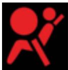
This indicator light should come on briefly when you first start your engine. If all airbags are working properly, the indicator light should go off after a few seconds. If the light stays on or comes on while driving, there may be a problem with your airbags. Take your vehicle to a service center to have them repaired.
